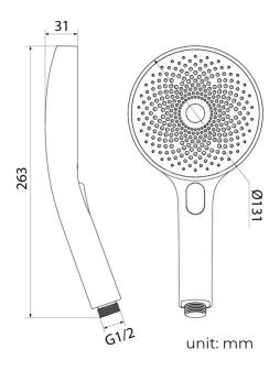
Flow Rate: 2.0 GPM / 7.6 LPM
